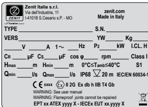
Silver sticker. Reproduces the pump nameplate.
